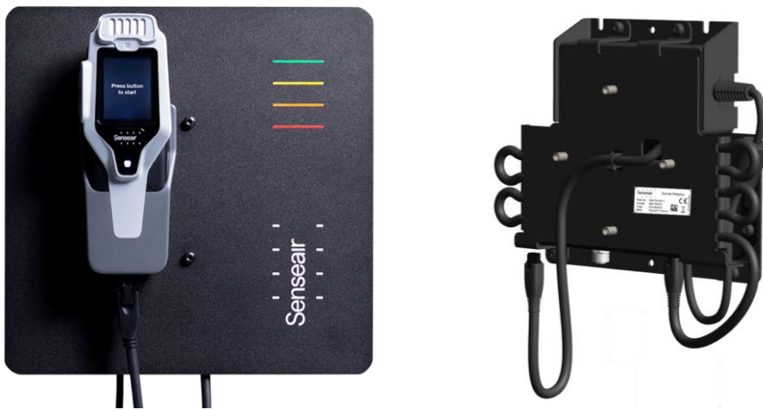
Figure 1 Senseair Workplace with and without the front plate. The label is attached behind the front plate.
