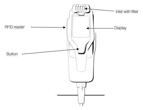
Senseair Workplace is an indoor¹ alcohol detector that accepts an exhaled breath sample and measures the concentration of alcohol, BrAC², in that exhaled breath sample³. The breath sample is provided without a mouthpiece. The Senseair Workplace is a calibration free device without limit on number of tests⁴.
