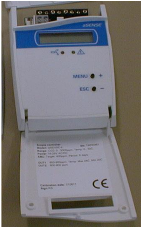
Figure 14 The aSENSE VAV with LEDs, push buttons and display
