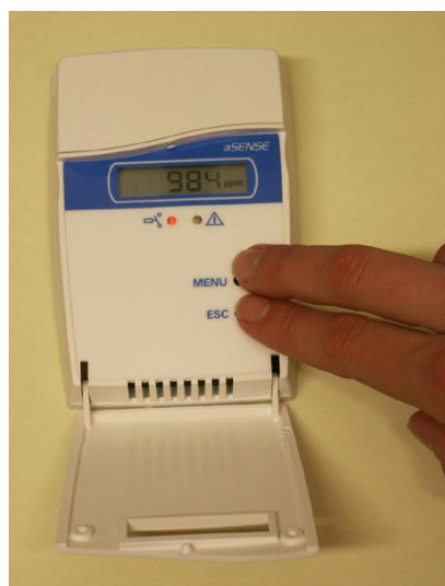
Figure 11 The ENTER command is done by pushing buttons MENU and ESC at the same time for about 14 seconds
