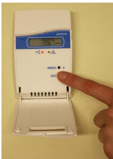
Figure 10 The push button MENU is pushed
