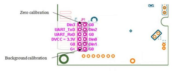
Figure 6. Senseair K33 ICB (component side) zero and background calibration inputs for calibration jumpers.
