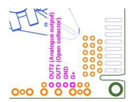
Figure 4. Senseair K33 ICB (OBA side) G+, GND, OUT1 and OUT2, 2.54mm hole spacing
