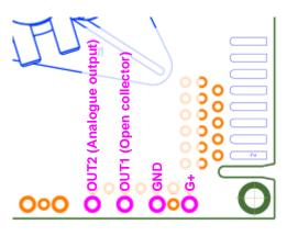
Figure 3. Senseair K33 ICB OBA side) (G+, GND, OUT1 and OUT2, 5.08mm hole spacing
