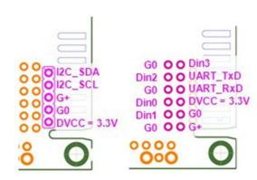
Figure 2. Senseair K33 ICB (OBA side) UART and I<sup>2</sup>C connections
