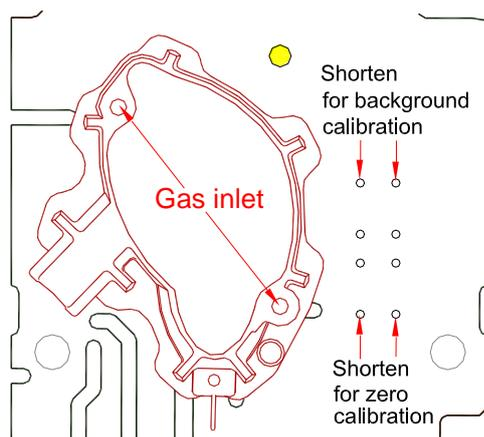
Figure 3 Holes to shorten for calibration
