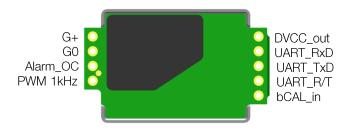
Figure 2. Pin assignment
