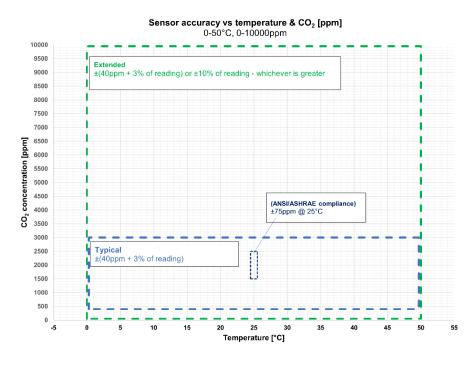
Figure 4. Accuracy over complete operating range (temperature and measurement of CO<sub>2</sub>).
