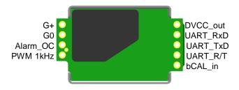
Figure 2. Pin assignment
