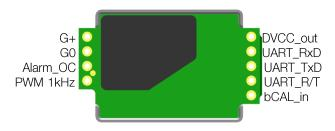
Figure 2. Pin assignment
