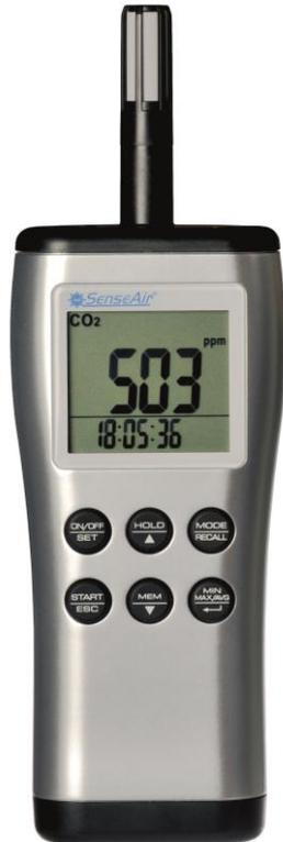
**pSENSE II™** is a hand-held and portable data logger, with rechargeable batteries and power adaptor. The instrument displays and records temperature, relative humidity, CO<sub>2</sub>, and calculates parameters such as dew point and wet-bulb temperature.
