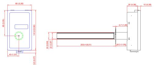
Dimensions of sensor in mm and inches
