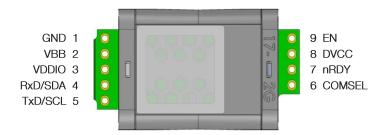
Figure 2 Pin configuration (top view)
